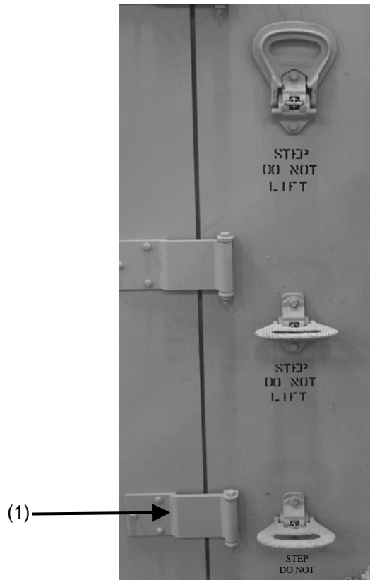
Figure 4-56. Main door hinges and utility steps.
