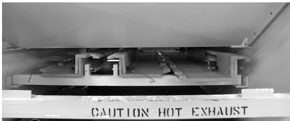
Figure 2-32. Nested detent rails stored above generator.
