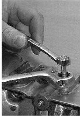
Figure 4-61. Loosening of hex nut.
