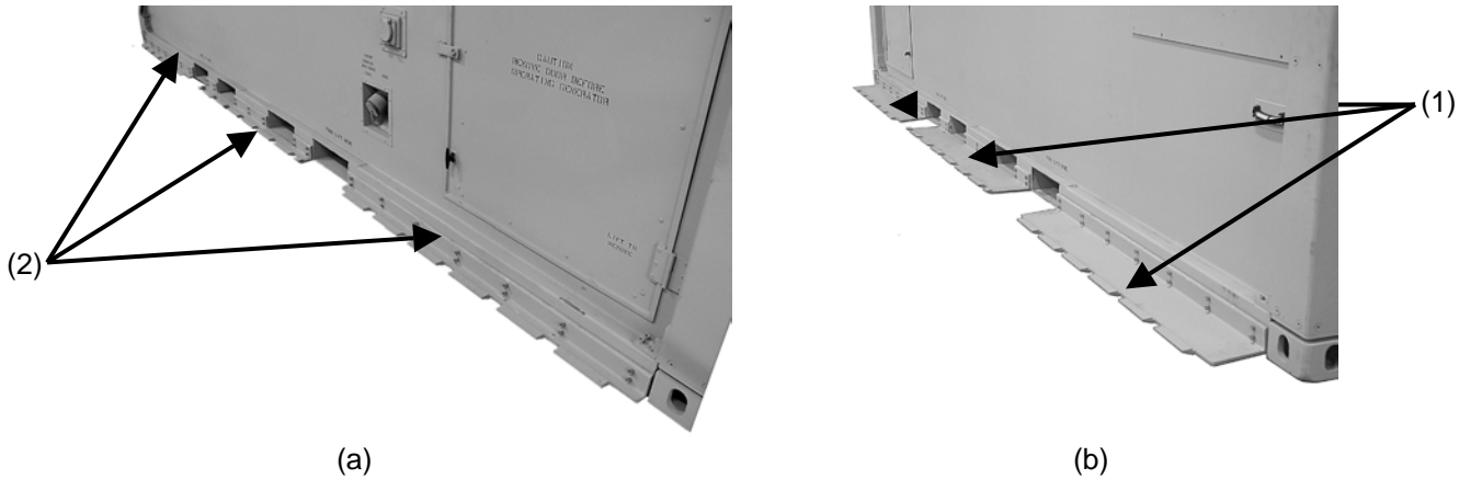
Figure 2-29. Detent rails installed on container.
